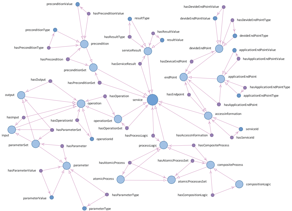
Figure 6.1: Semantic digraph of pervasive in-network service modelling and composition.
